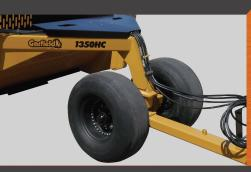
Gooseneck design allows good view of the cutting edge from the cab of the tractor.
