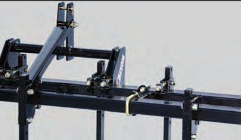
Easy adjustment for desired cultivation width, just slide the shanks on the tool holder bars.
