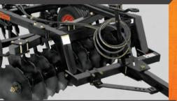
The frames for the different sections are made with tubular structural steel. It offers strong resistance to torsion and stability during work and transportation.
