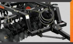
The frames for the different sections are made with tubular structural steel. It offers strong resistance to torsion and stability during work and transportation.
