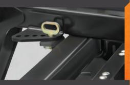
Qith five positions for the attack angle in both sections of the disc, which allows a fine flawless harrowing in any type of land.
