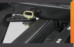
Up to 5 configuration positions for the attack angle in both front and rear disc sections allow flawless harrowing in any kind of terrain.
