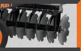
The bearings bathed in oil requirees less maintenance than greased bearings, Its double bearing oarlocks makes the implement structure more resistant than the conventional disc bearings.
