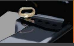
3 to 5 angle attack adjustment positions on front and rear disc sections, allowing flawless harrowing in any kind of soil.
