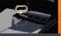
3 to 5 angle attack adjustment positions on front and rear disc sections, allowing flawless harrowing in any kind of soil.
