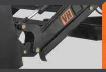
Attachment dump linkage provides greater attachment roll-back and dump angle.
