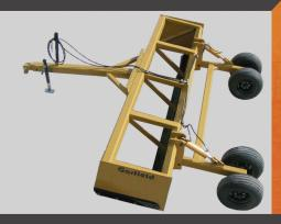
All units have a 3/8 step broke moldboard which alows material to roll instead of push it.
