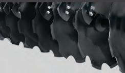
Multi-tillage system: with only one machine you can prepare the seedbed while mixing the residue, breaking up the toposil, and shattering the compacted subsurface layers.
