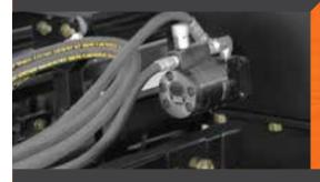
Adjustable brakes for plastic and irrigation hose holders. Opener - furrow grid to place the edge of the plastic.
