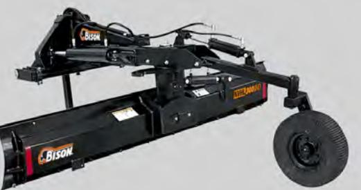
The heavy-duty design and construction of the NVHL Series make them ideal for the most rugged grading jobs. The 8, 9 and 10-foot moldboards are reinforced to withstand the most demanding conditions and can be reversed for backfilling. This top-of-the-line blade is rated for use on tractors up to 160 (2 WD) horsepower and features optional hydraulic controls for precision blade adjustment.
