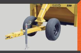
Heavy duty dolly reduces load on tractor and provides more flotation.
