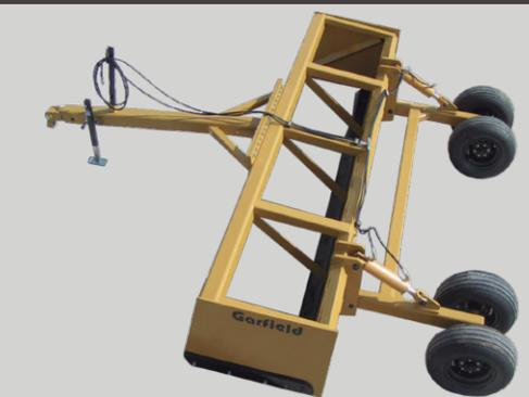
All units have a 3/8 step broke moldboard which allows material to roll instead of push it.
