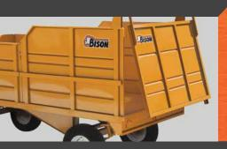
High clears axle, with reinforced lance and fifth wheel that covered the complete main frame, for a better load and transport stability.
