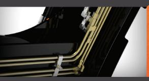
Hidden tubing under loader arms prevent exposure to shocks and provide a better location for the hoses, also giving greater operator visibility.
