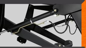
Double-acting cylinders made of highly durable chrome bar.
