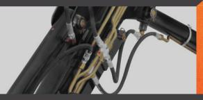
High burst pressure phosphatized hydraulic steel tubing and JIC no-leak fittings are standard.
