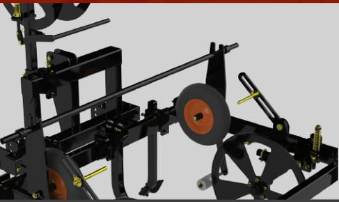
The greenhouse plastic mulch layer, pulls the irrigation belt and places the plastic for the padding in one step.
