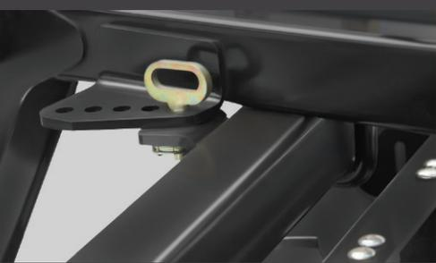
Up to 5 configuration positions for the attack angle in both front and rear disc sections allow flawless harrowing in any kind of terrain.
