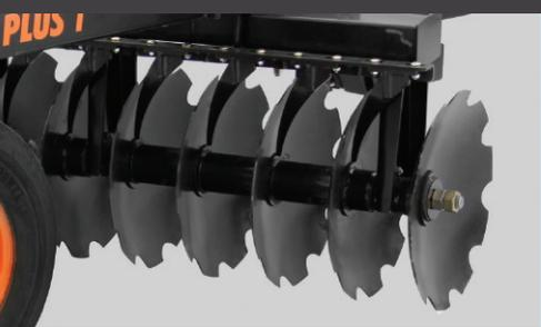
The bearings bathed in oil requires less maintenance than greased bearings, its double bearing oarlocks makes the implement structure more resistant than the conventional disc bearings.
