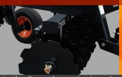
Used for soil preparation, controls undergrowth and allows fluid incorporation of residues.
