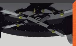
Four blades rotary cutter, causing a more effective and balanced cut. Such blades are not fixed, increasing the durability at the time of a blow.
