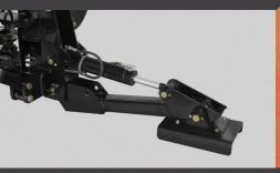
Standard stabilizer pads fit most applications and allow for greater machine stability. A safer operation results by avoiding sudden backhoe movements.
