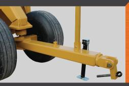
Dolly reduces stress on tractor and provides more flotation.
