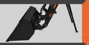
Attachment dump linkage provides greater attachment roll-back and dump angle. In addition, quick-attach compo-nents (except VH-900-ER) allow for easy mount and dismount in a matter of minutes.
