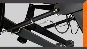
Double-acting cylinders made of highly durable chrome bar.
